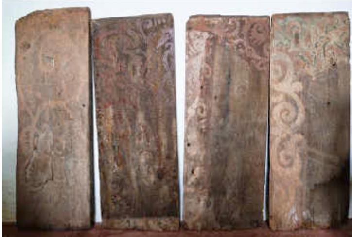
Figure 55 ~ Four panels currently stored in the vestry (above left) and the reverse of the far right two (right) showing rotten decay, dark staining and mould from damp and insect damage.
